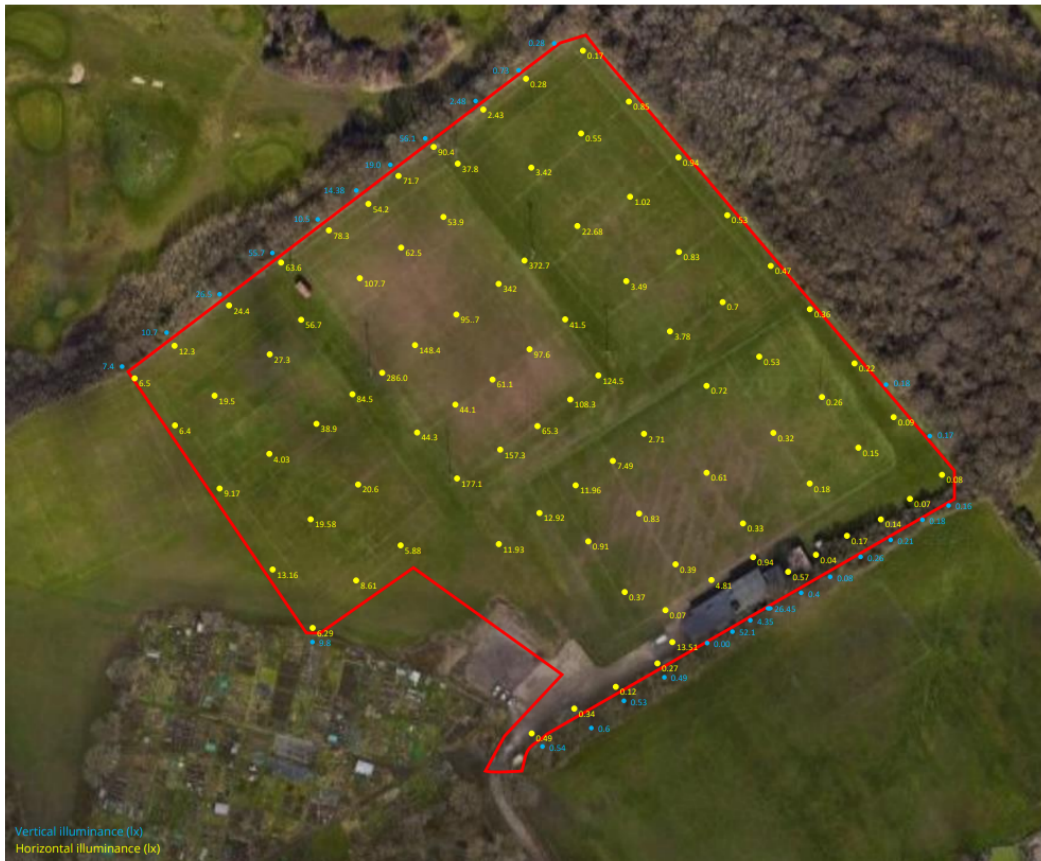
Existing lux level on site during night-time survey carried out by CPW at 22:30 on 12th July 2023.
